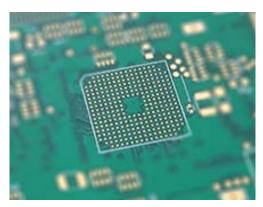
of pad size and spacing pitch. Secondly, the aspect ratio (depth to diameter) became limited by drill flute length, positional accuracy, rigidity of the tools (to prevent breakage), and the throwing power of acid copper plating systems. And lastly, the plating needed to close up the hole as much as possible, which led to problems with voiding, incomplete fill, and gas/solution entrapment.
