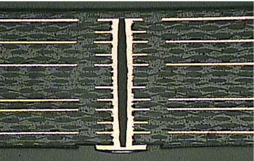
Figure 2 - San-Ei Kagaku PHP-900 Non-conductive Via Fill in Blind Via
